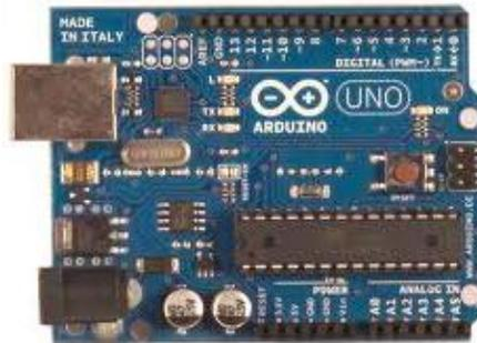
**Figura 40.** Tarjeta Arduino UNO.
