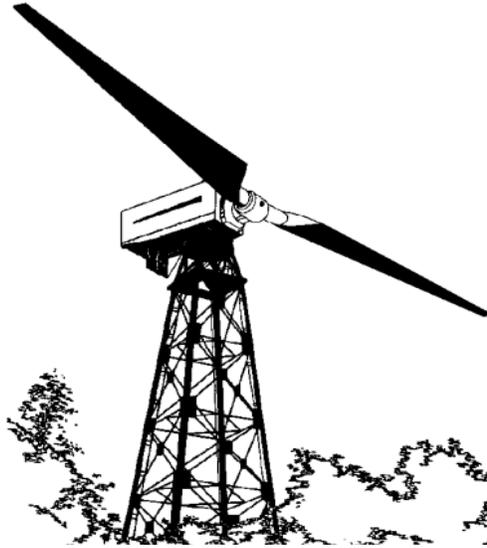
**Figura 2.8:** Aerogenerador experimental MOD-0A de 200 kW
