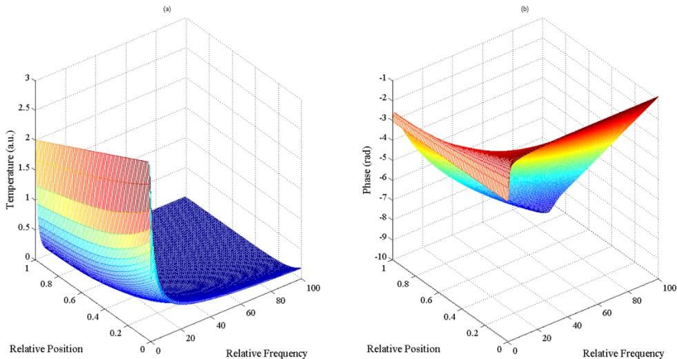
**FIGURE 4.** Calculation of: (a) Amplitude of the temperature variations, and (b) Phase of the temperature variations, as function of relative position and frequency. Robin boundary conditions were considered.
