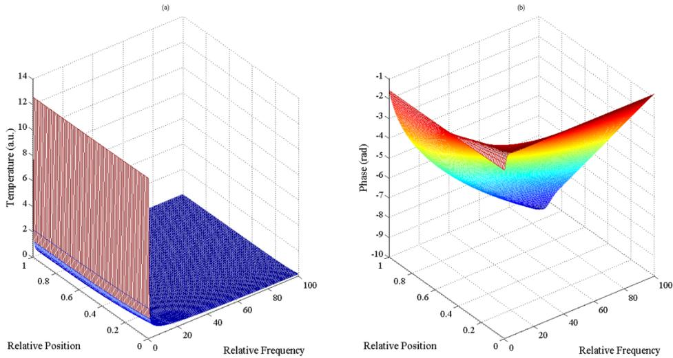
**FIGURE 3.** Calculation of: (a) Amplitude of the temperature variations, and (b) Phase of the temperature variations, as function of relative position and frequency. Neumann boundary conditions were considered.
