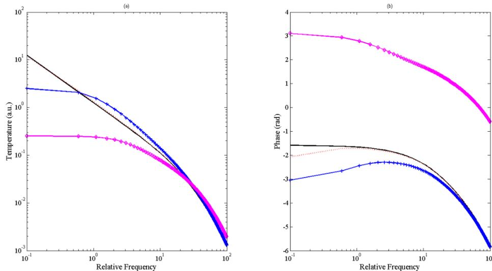
**FIGURE 5.** Comparison of the behavior of: (a) Amplitude and (b) Phase of the temperature variations as function of relative frequency, for sinusoidal wave modulation. The black line represents the solutions under Neumann boundary conditions. The calculations under Robin boundary conditions were performed for different values of  $Bi_s$ : 0.05 (red dotted line), 0.5 (blue line) and 5 (pink line).
