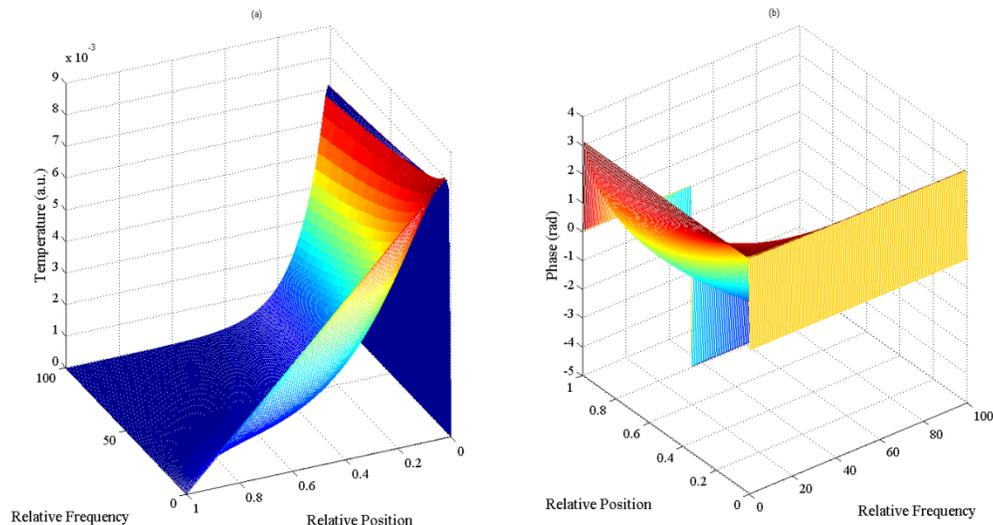
**FIGURE 2.** Calculation of: (a) Amplitude of the temperature variations, and (b) Phase of the temperature variations, as function of relative position and frequency. Dirichlet boundary conditions were considered.
