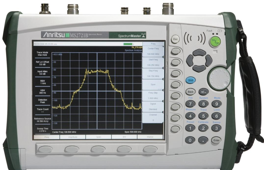
*Spectrum Master™ MS2721B Spectrum Analyzer*
