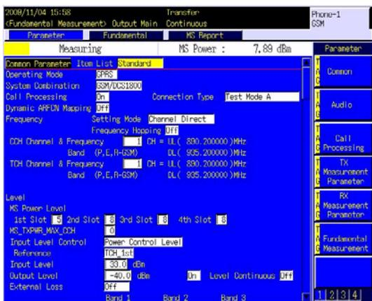
Figure 10. Power measurement
