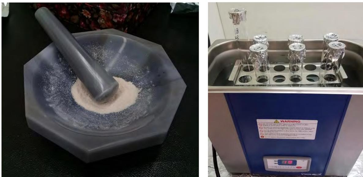
Figure 46: The two extraction equipment used to analyze the biopsies: mortar (left) and ultrasound bath (right).
