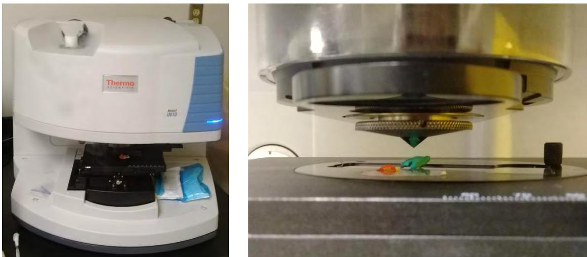
Figure 36: The  $\mu$ FT-IR used for the determination of the polymer of plastic debris.
