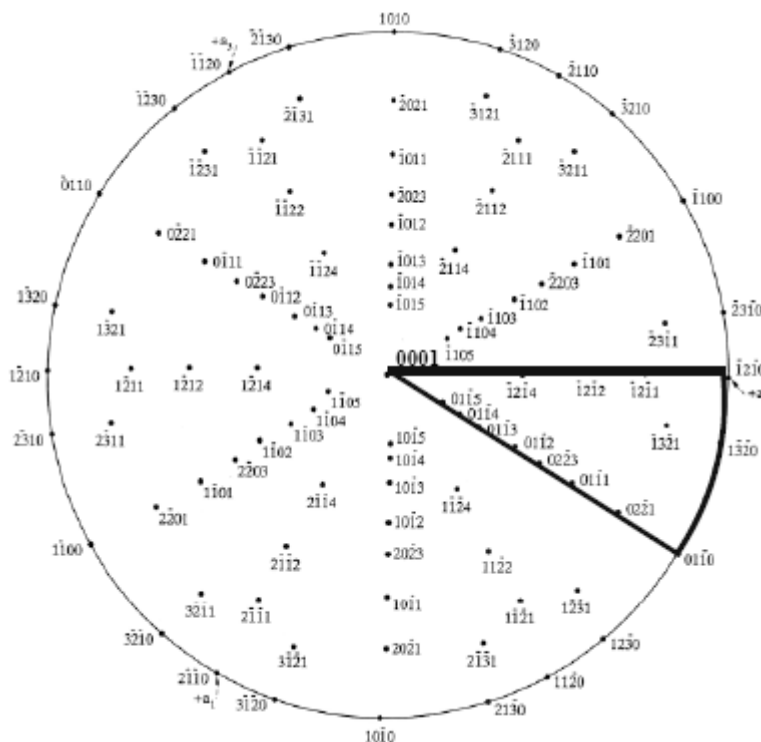
Fig. 4: Standard (0001) stereographic projection of an HCP crystal structure showing a diagrammatic illustration of the inverse pole figure (blue triangle) used in this study for the representation of textures in extruded profiles [24].
