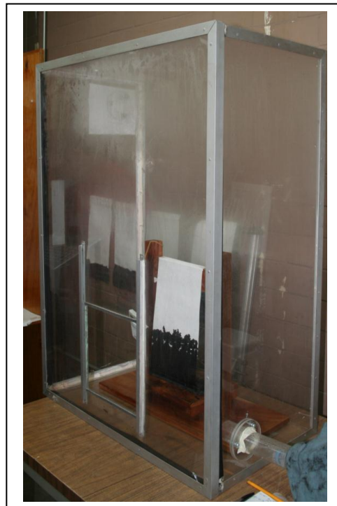
Figure 1. Device of the imbibition test, where the recipient with the fluid, the filter paper, the wooden frame, the humidity meter and the isolation chamber are shown.
