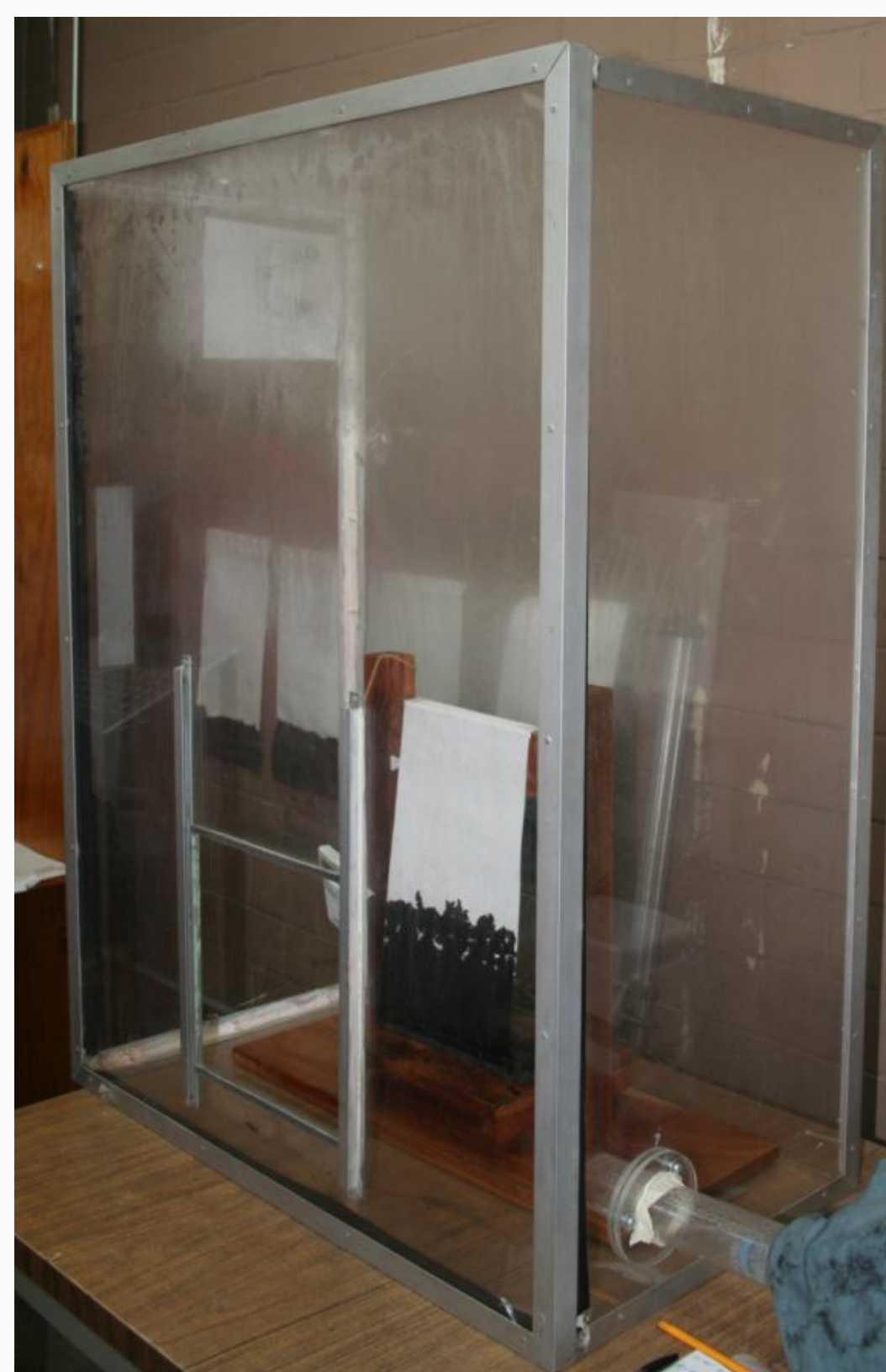
Figure 1. Assembly of the imbibition test, where the fluid, the paper, the wooden device, the meter of temperature and humidity, recipient that contains the fluid, as well as the transparent camera of isolation are shown.
