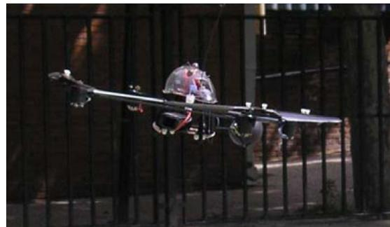
**Figura 3. Quad Rotor autónomo**
