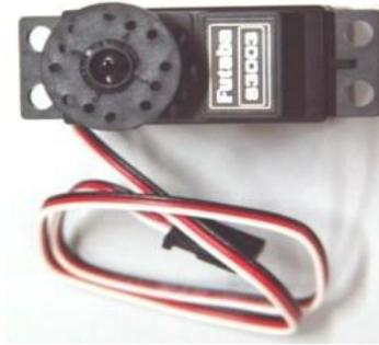
**Figura 6. Servomotor**
