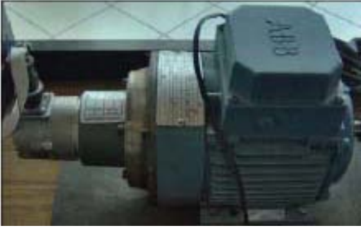
Fig. 4. Encoder coupled with the induction motor
