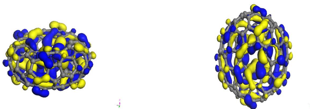
Figure 5 HOMO shapes and sizes for the C_{120} nanotorus. Contributions are larger from outer zone.
