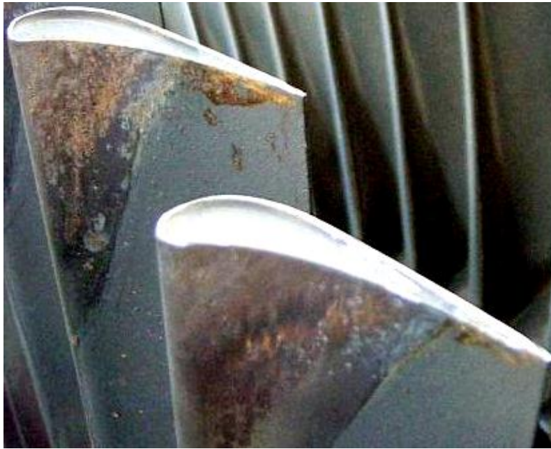
Figure I.3: Blades damaged by erosion in the low pressure section (Rueda, 2006).
