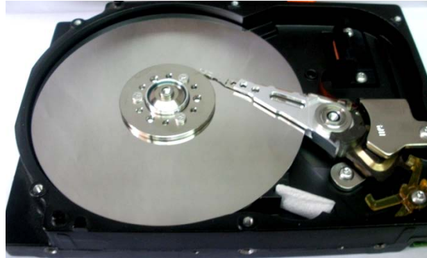
Figura A8.1. Headcrash no visible.
