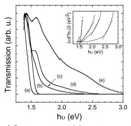
**Figure 4.** Room temperature transmission spectroscopy spectra for samples deposited at  $T_s = 600$  °C. (a) polycrystalline CdTe sample, (b) MY1, (c) MY5, (d) MY9 and (d) MY6. The inset corresponds to the fitting of the transmission spectra to the model of direct transitions between parabolic bands.
