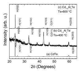
**Figure 2.** Representative X-ray diffractograms for (a) CdTe film, (b)  $Cd_{1-x}Al_xTe$  films deposited at  $T_s=400$  °C and (c)  $Cd_{1-x}Al_xTe$  films deposited at  $T_s=400$  °C.
