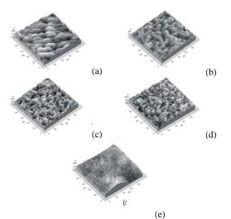
Figure 1. Atomic force micrographs for samples deposited at  $T_{\rm s}$  =400 °C . (a) CMT8, (b)CMT9, (c) CMT7, (d) CMT3 and (e) CMT5.
