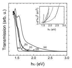
Figure 3. Room temperature transmission spectroscopy spectra for samples deposited at  $T_s = 400$  °C. (a) sample CMT5, (b) CMT9, (c) CMT3, (d) CMT8 and (e) CMT7. The inset corresponds to the fitting of the transmission spectra to the model of direct transitions between parabolic bands.
