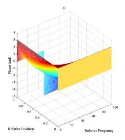
**FIGURE 2.** Calculation of: (a) Amplitude of the temperature variations, and (b) Phase of the temperature variations, as function of relative position and frequency. Dirichlet boundary conditions were considered.
