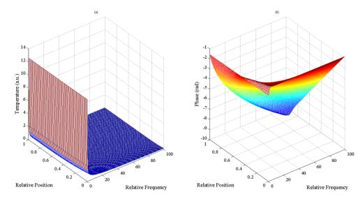
**FIGURE 3.** Calculation of: (a) Amplitude of the temperature variations, and (b) Phase of the temperature variations, as function of relative position and frequency. Neumann boundary conditions were considered.
