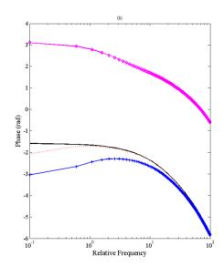
**FIGURE 5.** Comparison of the behavior of: (a) Amplitude and (b) Phase of the temperature variations as function of relative frequency, for sinusoidal wave modulation. The black line represents the solutions under Neumann boundary conditions. The calculations under Robin boundary conditions were performed for different values of  $Bi_s$ : 0.05(red dotted line), 0.5 (blue line) and 5 (pink line).
