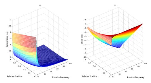
**FIGURE 4.** Calculation of: (a) Amplitude of the temperature variations, and (b) Phase of the temperature variations, as function of relative position and frequency. Robin boundary conditions were considered.
